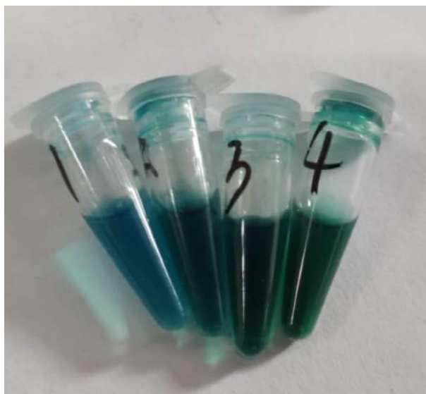
Figure 2: Color development of TMB induced by cerium oxide nanoparticles
