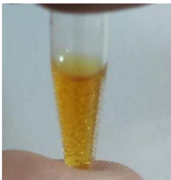
Figure 3: Rapid oxygen release from H 2 O 2 induced by cerium oxide nanoparticles
